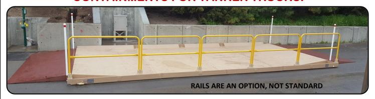
TRI-STAR MAX DRIVE-IN CONTAINMENT: Constructed of plate steel, and featuring rugged trilinear drive-over sidewalls, with a 62mil fiberglass protective coating and a non-slip grit surface. Modular design comprised of bolt together panels (ea. 7' x 13'W or 16'W) employing a semi-flush joint. Includes four 1-1/2" drain ports (one in each corner) and a ball valve and steel filter box. Anchor plates can be employed to secure system to substrate.
