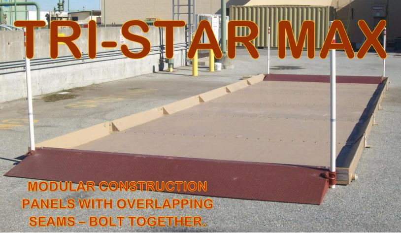
(Pictured Above) Tri-Star MAX Containment Pad configured for the 2,500g 978 HEMTT refueler. System Dim. 42' long by 13' wide by 9" high, Capacity – 2,850g (110% of refueler). Entry ramp extends 3' outside and 3' inside the sump end wall. Interior half of ramp is integral to sump.
